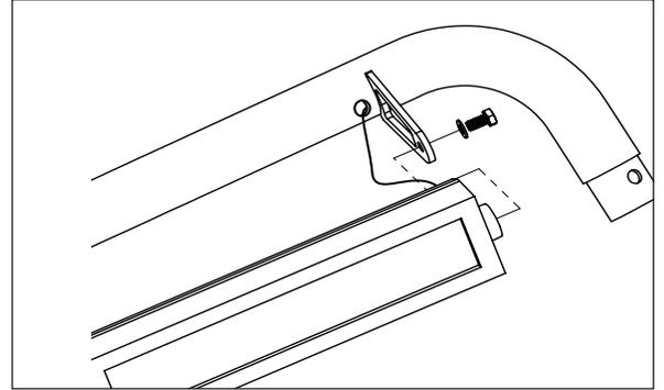
2. Attach LH and RH brackets to crossbar with supplied M8 button head bolt and M8 lock nut. Do not tighten completely to allow for adjustment.
